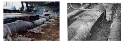
Figure 2: Buried pipelines under earthquakes - ductile iron pipes with seismic joints surviving large permanent ground deformation (left) and brittle failure of cast iron pipes (right)
